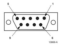
Figure 2-6. 9-Pin D-Sub Connector
